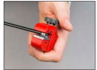
Positioning of line to scrape the covering
